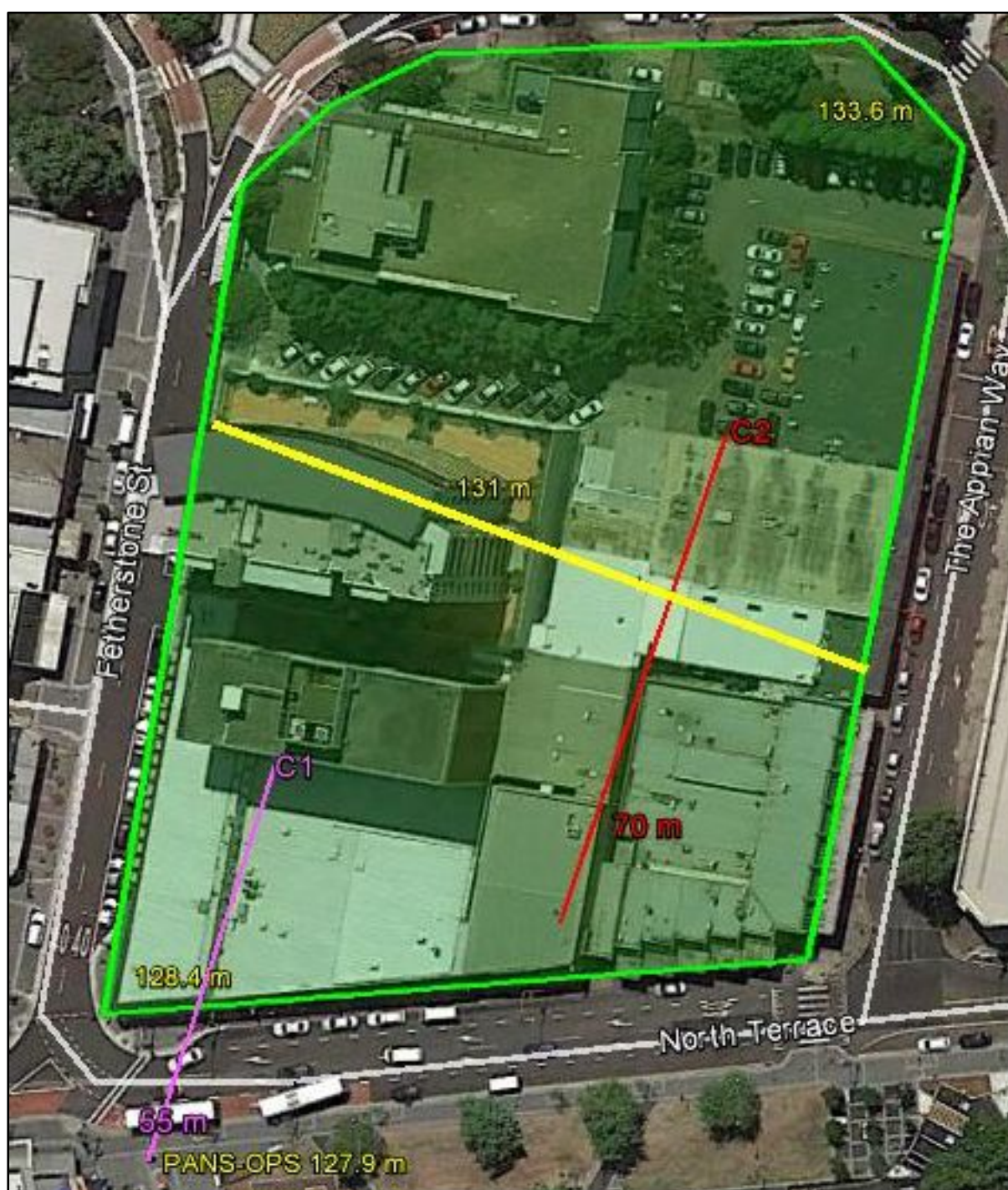
Figure 6.6 Crane and jib locations and the PANS-OPS surfaces
