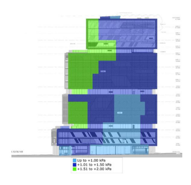
Figure 1b: Positive Peak 1000 year return period Ultimate Net Pressure Zone Diagram – East Elevation
