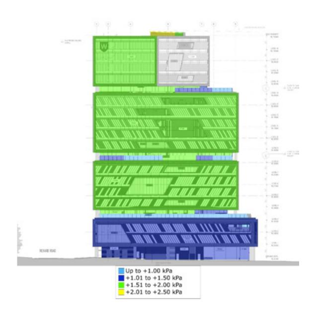
Figure 1d: Positive Peak 1000 year return period Ultimate Net Pressure Zone Diagram – West Elevation
