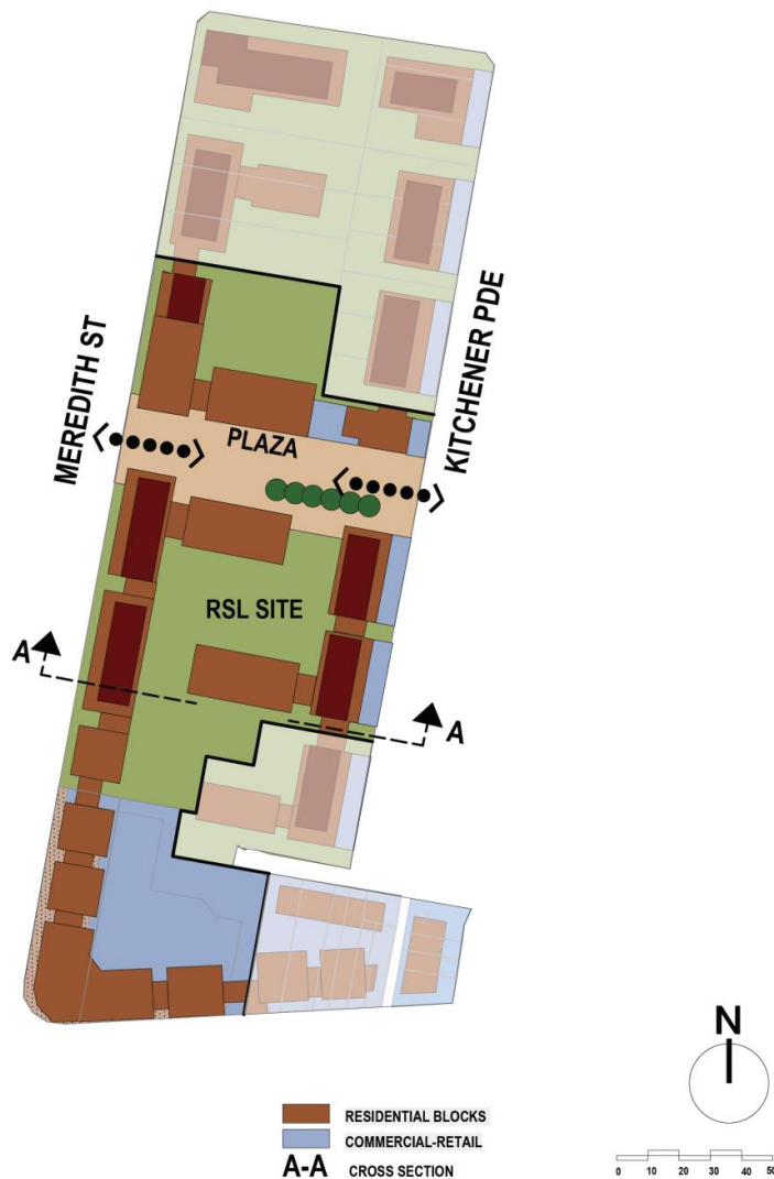
Figure 3e: Proposed building envelope for mixed use development on this key strategic site (refer to cross-sections for appropriate number of storeys)
