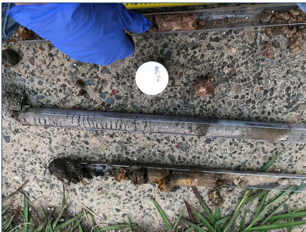
Photograph 7: Push tube samples in BH11 into the soil/rock interface – hydrocarbon impacted clay down to natural clays.
