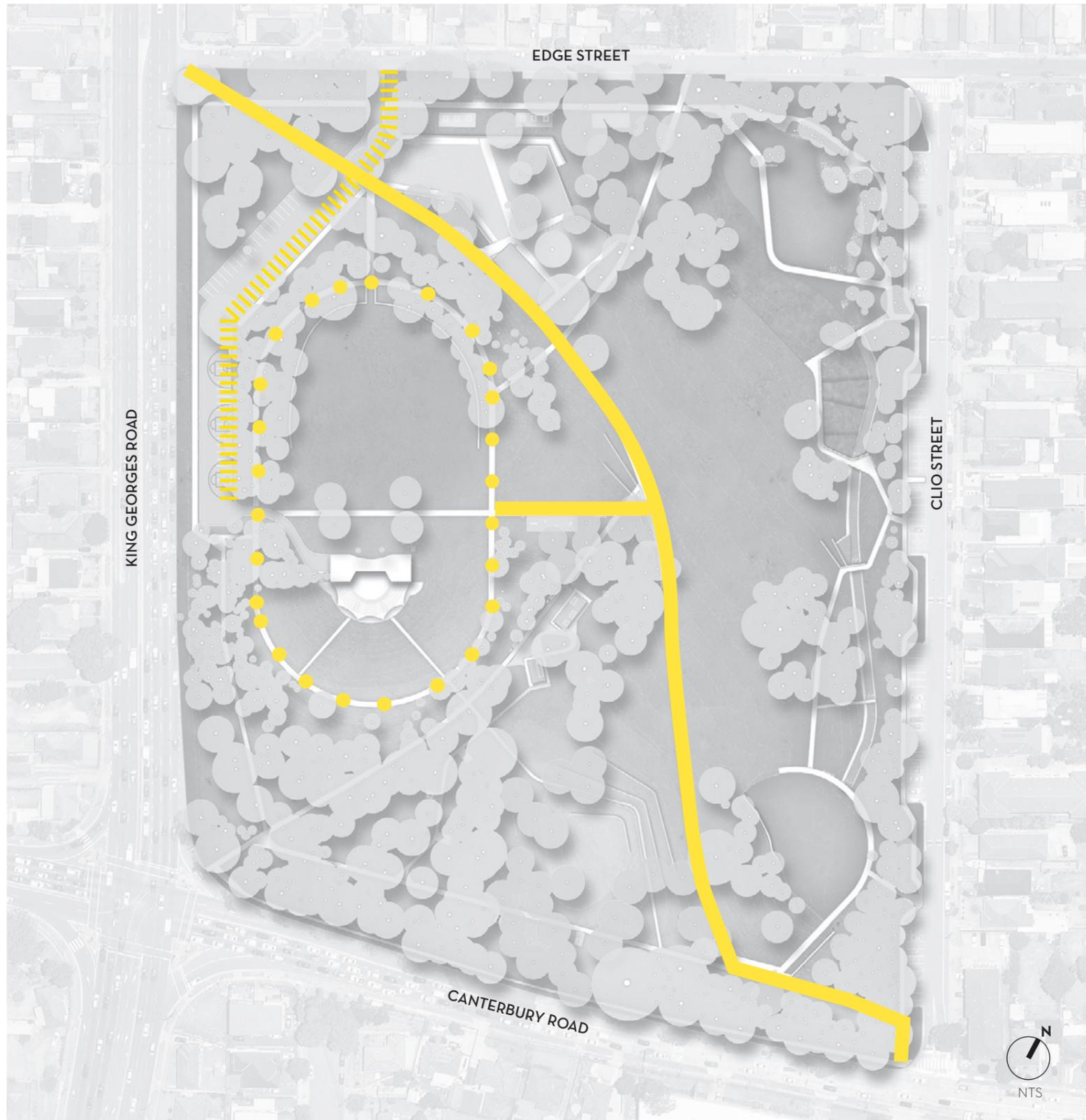
New post top lighting is proposed to the primary path, the diagonal path connecting from the western corner of the park at Edge Street, to the eastern corner of the park at Clio Street. Flood lights are proposed in the western carpark, and around the field to allow for night time sports use.
